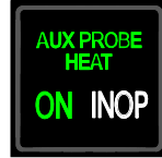
Figure 1-170. Independent Pitot/AOA Probe Auxiliary Heaters Error Detected
