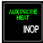
Figure 1-169. Independent Pitot/AOA Probe Auxiliary Heaters Inoperative or Manually Switched Off
