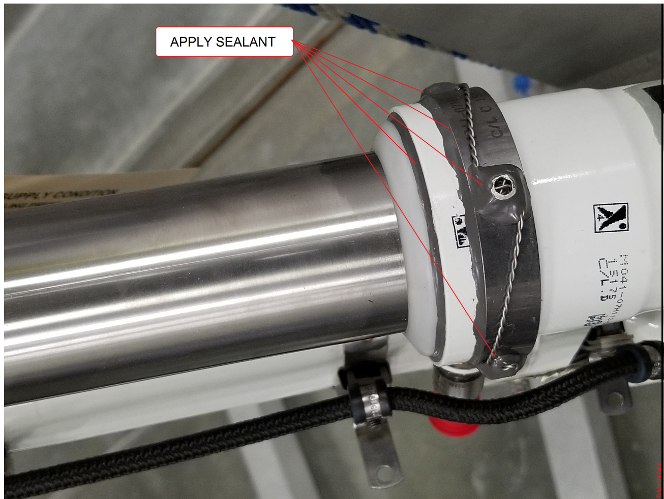
Sealant Application Figure 803 (Sheet 2 of 2)
