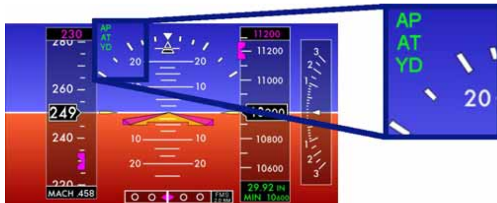
Figure 15-3. Autopilot and Yaw Damper Engaged Indications – PFD
