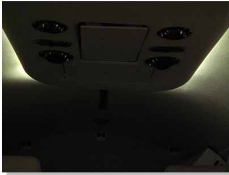
Figure 10-7. Overhead Cabin Wash Lighting
